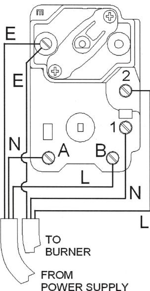
SECURE ALL THE LIVE AND NEUTRAL WIRES TOGETHER WITH CABLE TIES, KEEPING THE CABLE TIES AS CLOSE TO THE LIVE CONNECTIONS, B AND 2, AS POSSIBLE
