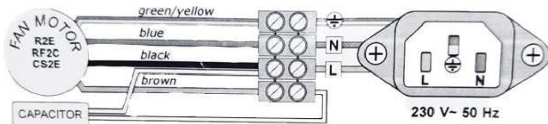
Connecting cable should be 3 x 0.75 mm<sup>2</sup> in cross-section area (3x20 AWG).
