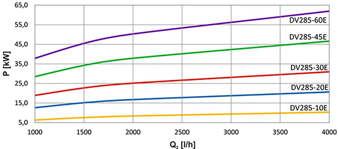
DV285E –  $\Delta T = 10 \text{ K}$  –  $Q_1 = 2400 \text{ l/h}$  – water/water
