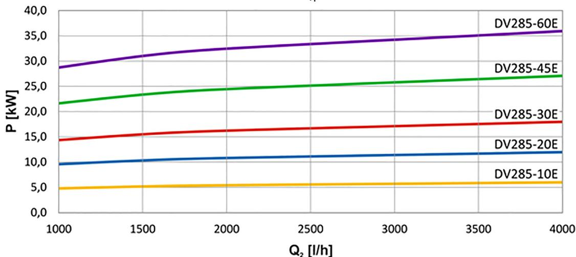
DV285E –  $\Delta T = 10 \text{ K}$  –  $Q_1 = 1500 \text{ l/h}$  – water/water
