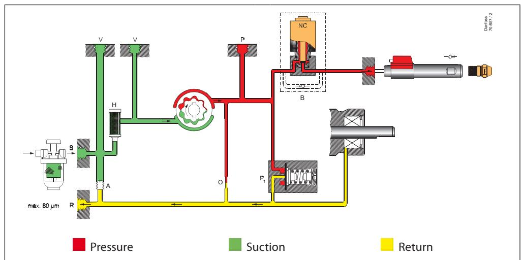
Before the burner starts the oil is heated in the oil preheater and in the nozzle line. This causes the oil to expand. The safety shut-off valve in the preheater prevents the oil from dripping out of the nozzle because the check valve B in the solenoid valve opens and thus makes a connection to the return or suction side of the pump.
