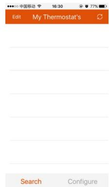
Note: WiFi name can't include the sign “—” and “\_”, WiFi from router must be 2.4G, 4G wifi from the other mobile phone hotspots is also ok, 5G router wifi is not ok.
