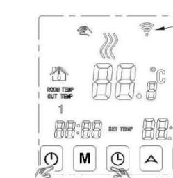
8.Press start connection on the phone,if thermostat and the mobile phone connection is success, the WiFi icon will stop flashing
