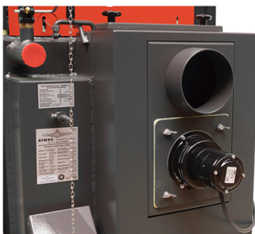
Exhaust fan and flue gas neck
