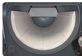
Combustion chamber with ceramic fittings
