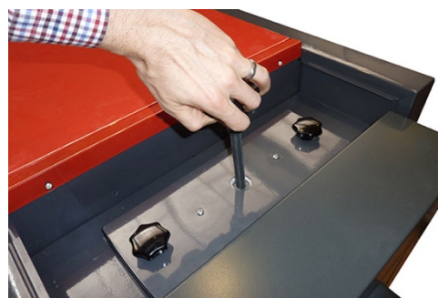
Demonstration of operational cleaning of a tube heat exchanger
