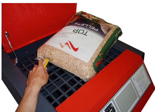
Example of standard refilling of pellets from 15 kg bags
