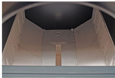
Combustion chamber with heat-resistant fitting – nozzle
